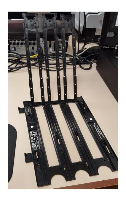
4. Beginning at the top tray, insert your negative filmstrips into the tray. The numbers on the filmstrips should be facing up towards you. Slide the left edge of the filmstrip under the two tabs in the tray to hold in place.
