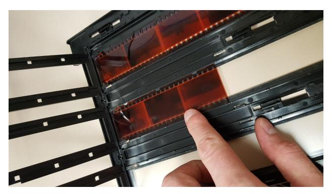
6. Next, secure the filmstrips in place by closing the three tabs. Press all around so the entire sockets on the side of the tab to lock negatives into place.
