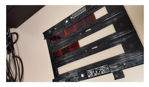
7. Next, flip the negative adapter over, and line up the two small feet on the bottom left side of the negative adapter with the two openings on the scanner bed (by the two white triangles. (The white triangles on the adapter will line up with the ones on the scanner when installed correctly)
