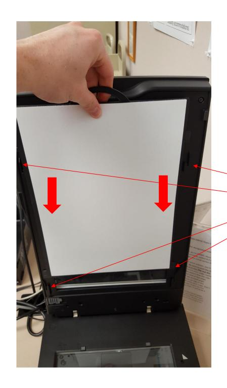
Line white cover above the four tabs, then push down to secure.
