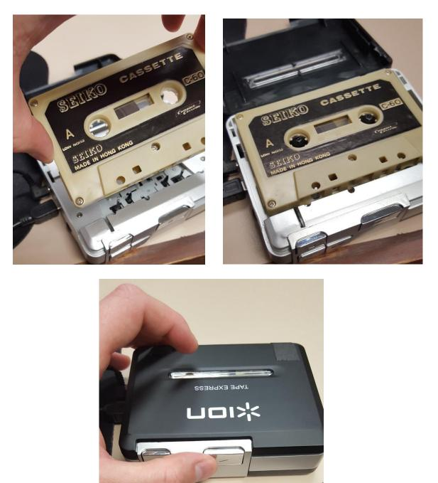
3. If needed, press the REWIND BUTTON on the ION cassette converter to rewind your tape.
