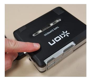
5. If needed, press the <u>REWIND button</u> to rewind the tape to the start. Press the <u>STOP</u> <u>button</u> once the tape has finished rewinding.
